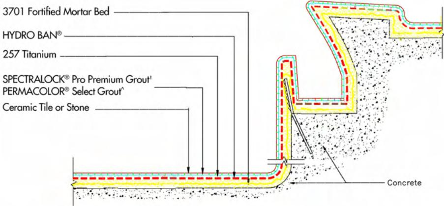
Note: Slurry Bond Coat of 257 Titanium is required under the mortar bed at all horizontal surfaces.
