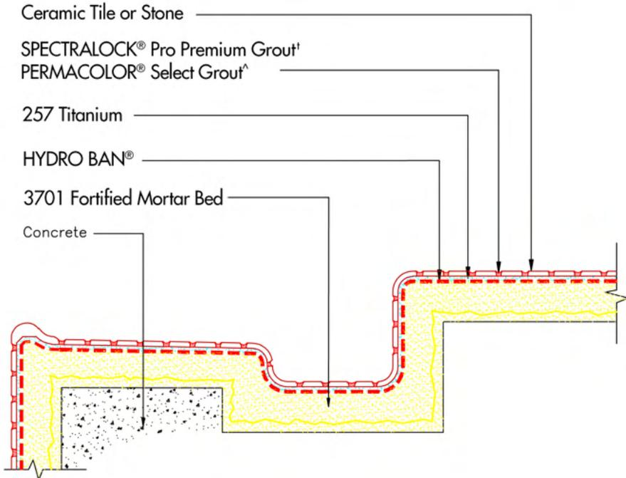
Note: Slurry Bond Coat of 257 Titanium is required under the mortar bed at all horizontal surfaces.
