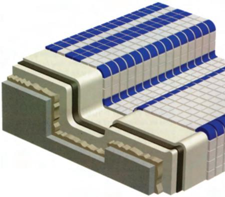
Figure 8.3 – Thick Bed Floor / Waterproofing System with drain detailing.
