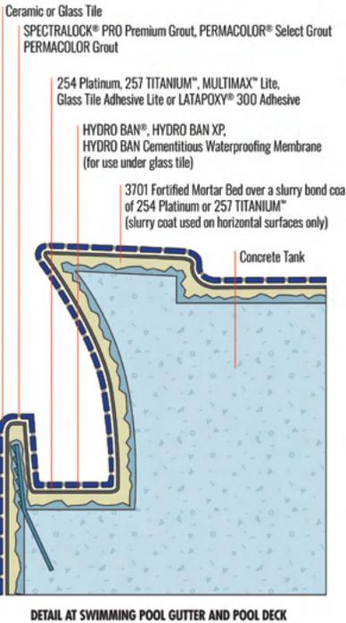
**DETAIL AT SWIMMING POOL GUTTER AND POOL DECK**
