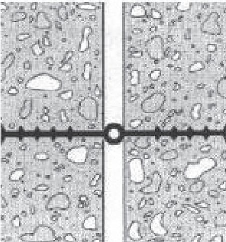
Figure 4.3 – Typical shape and placement of water stop where floor and wall join in pool movement joint.<sup>6</sup>
