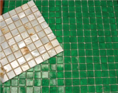
Figure 5.4 — Two examples of paper-face mounted glass mosaic tile.
