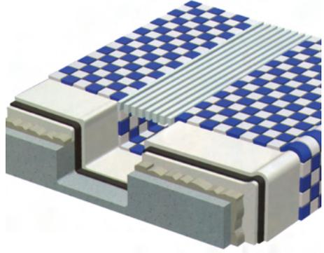
Figure 8.4 – Tiled pool deck trench drain and pool tank transition.
