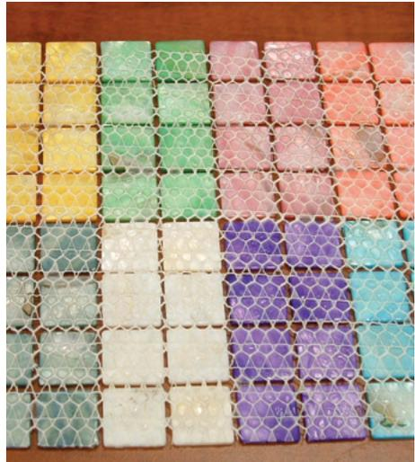
Figure 5.7 — An example of rear mesh mounted glass mosaic tile.
