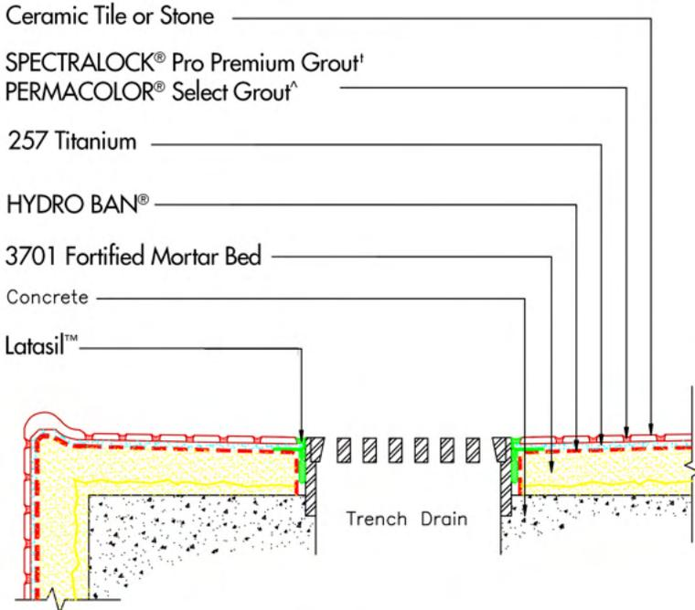
Note: Slurry Bond Coat of 257 Titanium is required under the mortar bed at all horizontal surfaces.
