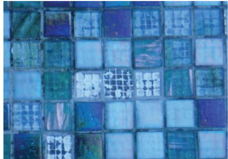
Figure 12.10 – The effects of a mesh mounted glass tile utilizing an adhesive and mesh that are not suitable for continuous submersion. The adhesive has expanded and lost bond to the back of the tiles.
