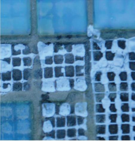
Figure 5.9 – A classic example of an improper adhesive used to mount the mesh for submerged installation. The adhesive has changed color from clear to white and has swelled significantly, forcing delamination.
