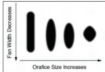
Figure 6.21 — The example demonstrates the spray pattern of new and worn spray tips. As wear occurs, the pattern size decreases and the orifice size increases. As a rule of thumb, it is best to replace the spray tips after spraying 30–45 gallons (114–171 liters) of HYDRO BAN® or HYDRO BAN XP.
