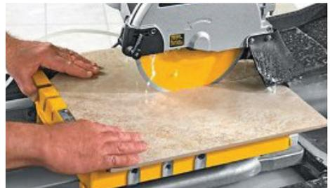
Figure 6.10 — A commercial grade wet saw is ideal for cutting all types of tile and stone in swimming pool, fountain or water feature applications.
