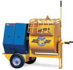
Figure 6.9 — Rotating Blade Type Mixer.
