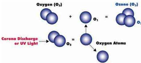
Figure 11.1 – Diagram of how ozone is created by an ozone generator.
