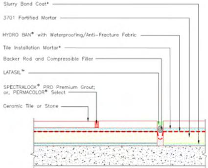
Figure 7.18 – Profile view detail depicting the waterproofing membrane looped into the movement joint.
