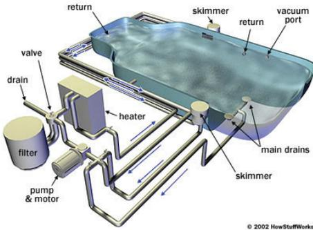
Figure 4.6 – Cut away view of a typical pool pump and filtration system.<sup>7</sup>
