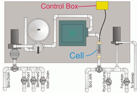
Figure 11.2 – A typical salt water circulation and treatment system4.
