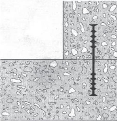
Figure 4.2 – Typical shape and placement of water stop where floor and wall join in pool construction.<sup>5</sup>
