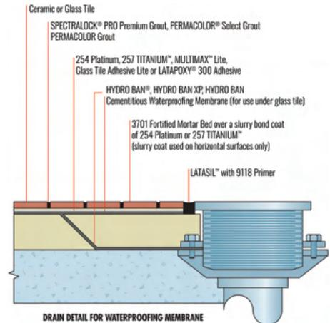
Figure 7.21 – Thick Bed Floor / Waterproofing System with drain detailing.
