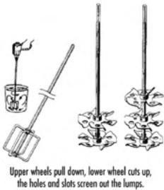
Figure 6.8 — Variety of Mixing Paddles used for Drill Type Mixers.
