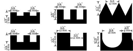
Figure 6.11 – Notched trowel sizes for installation of adhesive mortars.
