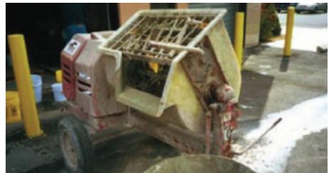
Figure 8.3 – Rotating blade type mixer.
