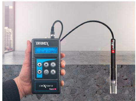
Figure 2.17 – In Situ Moisture Testing.
