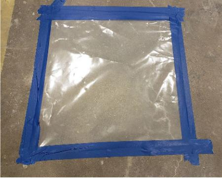
Figure 2.18 — ASTM D4263 — Plastic Sheet Method — 18" x 18" (45 cm x 45 cm) sheet of plastic is tightly taped to the substrate and allowed to sit undisturbed for 24 hours. If water or condensation is observed, then a measure of moisture vapor transmissions is present. This test will not provide a quantitative moisture vapor emission rate.
